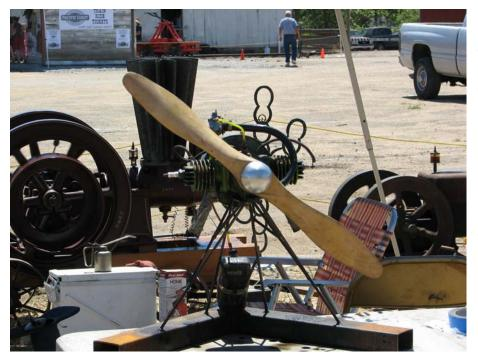
Here's an opposed twin I saw last month at a big convention of "hit and miss" engine guys. That prop is about two feet in diameter, and the engine looked too old and gutless for a man carrying ultra light, but too big for a giant scale ship. It took a while to find the owner, but I had to know. It turns out to be an old Maytag washing machine engine with a hand carved prop.
