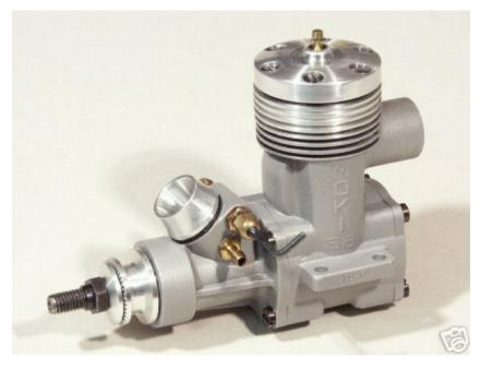
This Moki Schnuerle has three bypasses. The larger one is in the same place on the left side as the engine above. There are also two extra bypasses called boost ports fore and aft. The forward one is visible in the picture. The main bypass on a Schnuerle doesn't shift if the exhaust direction shifts. That's because the main bypass entry would be partly masked by the crank web. The boost port intakes sit higher in the sleeve and are above the crank web.
